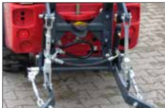
Three point connection system
