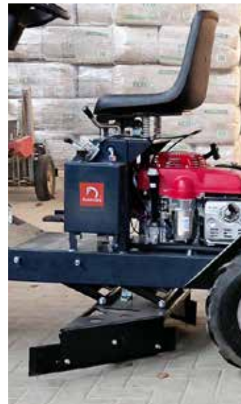
spring-mounted driver's seat
