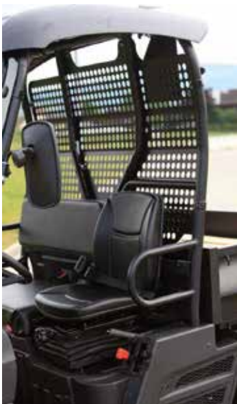
Rain-Sunshine-Roof, spring-mounted height-adjustable seat, windshield incl. wiper and washer
